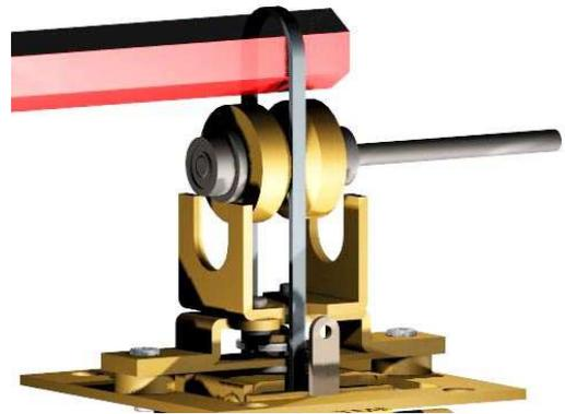
The Top Pulley is not fastened into the UPM2 frame in any way, it is simply held in place by the tension of the drive belt. This is quite intentional.
