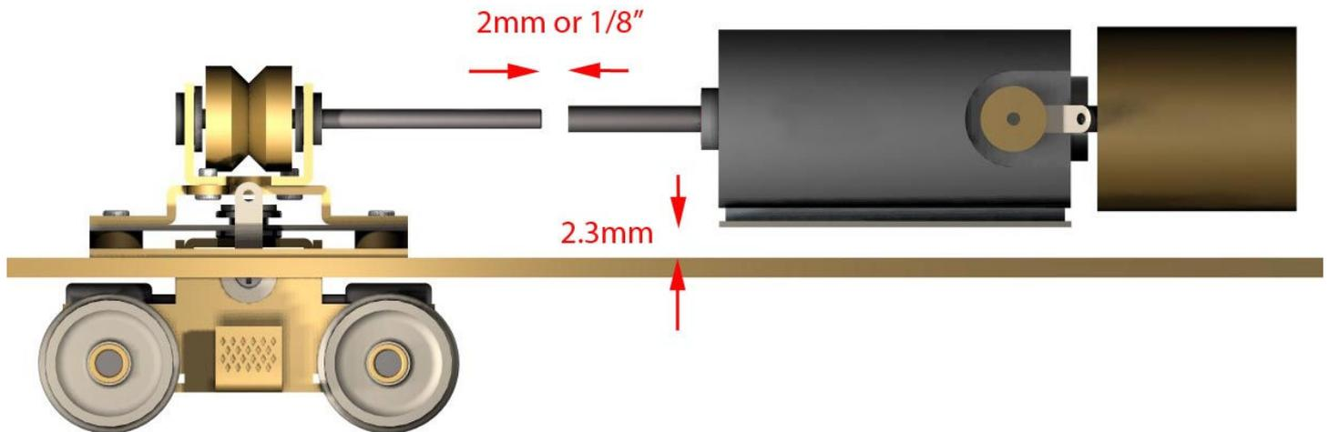
To pack the motor up to the right height, pieces of Evergreen styrene can be used, perhaps glued to the floor of the model, then the motor assembly can be attached using the four small self-tapping screws.
