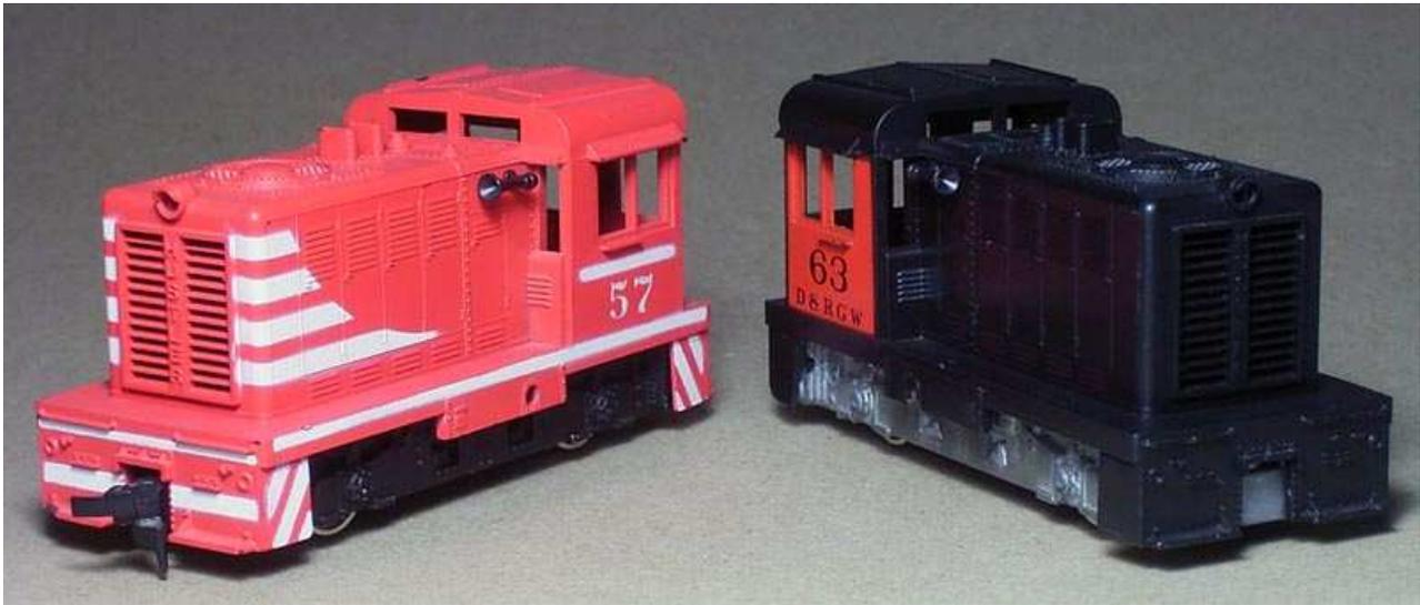
The First Generation model, shown on the right above, is the easiest model to convert. To begin, remove the body by popping it off the round lugs on the side of the cast Mazak frame.
